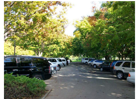
FIG. II.A.3: LANDSCAPED PARKING A planted area located between parking stalls provides space for canopy trees to shade cars and reduce the parking lot's heat island effect.
