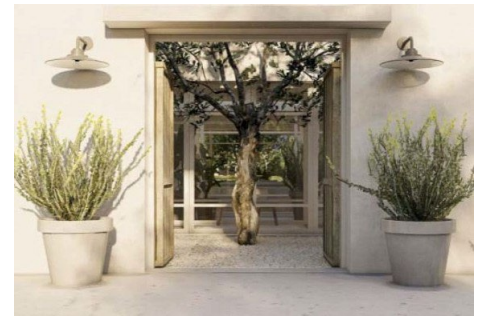
FIG. II. F.3: DOWNWARD LIGHTING Low profile lanterns direct light downwards to reduce light pollution on site.
